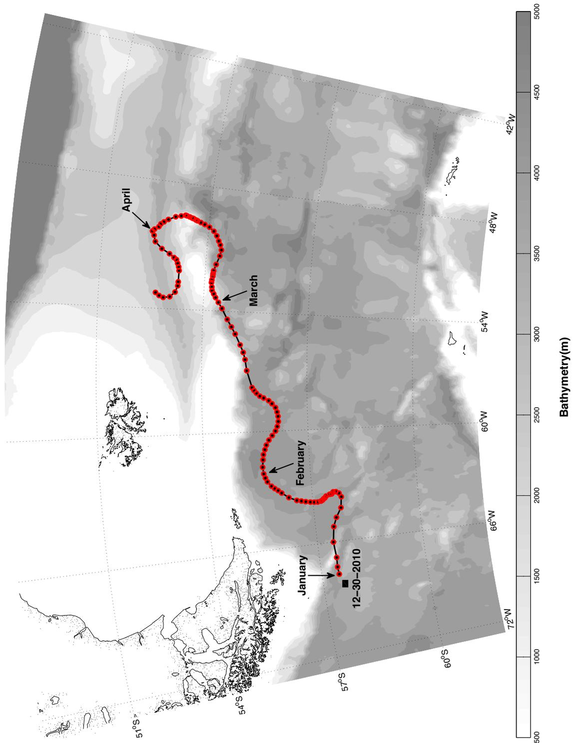
Figure 1. APEX 4782 track diagram from GPS position data. Red dots indicate CTD profiles with GPS positions, whereas the black square is deployment position (with date). Bathymetry is shaded in 500-meter intervals, according to the color bar.
