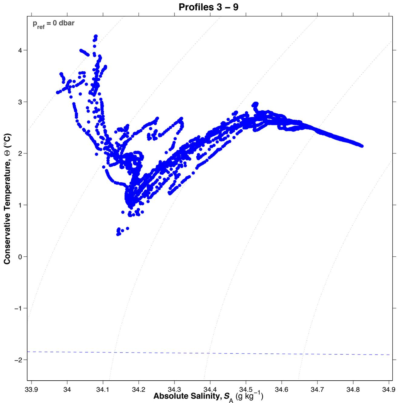
Figure 4: Conservative Temperature ( $^{\circ}\text{C}$ ) versus Absolute Salinity ( $\text{gkg}^{-1}$ ) along track, starting with the first profile after deployment, for APEX 4779. Each figure shows seven successive profiles. The freezing line is indicated by the blue dashed line.
