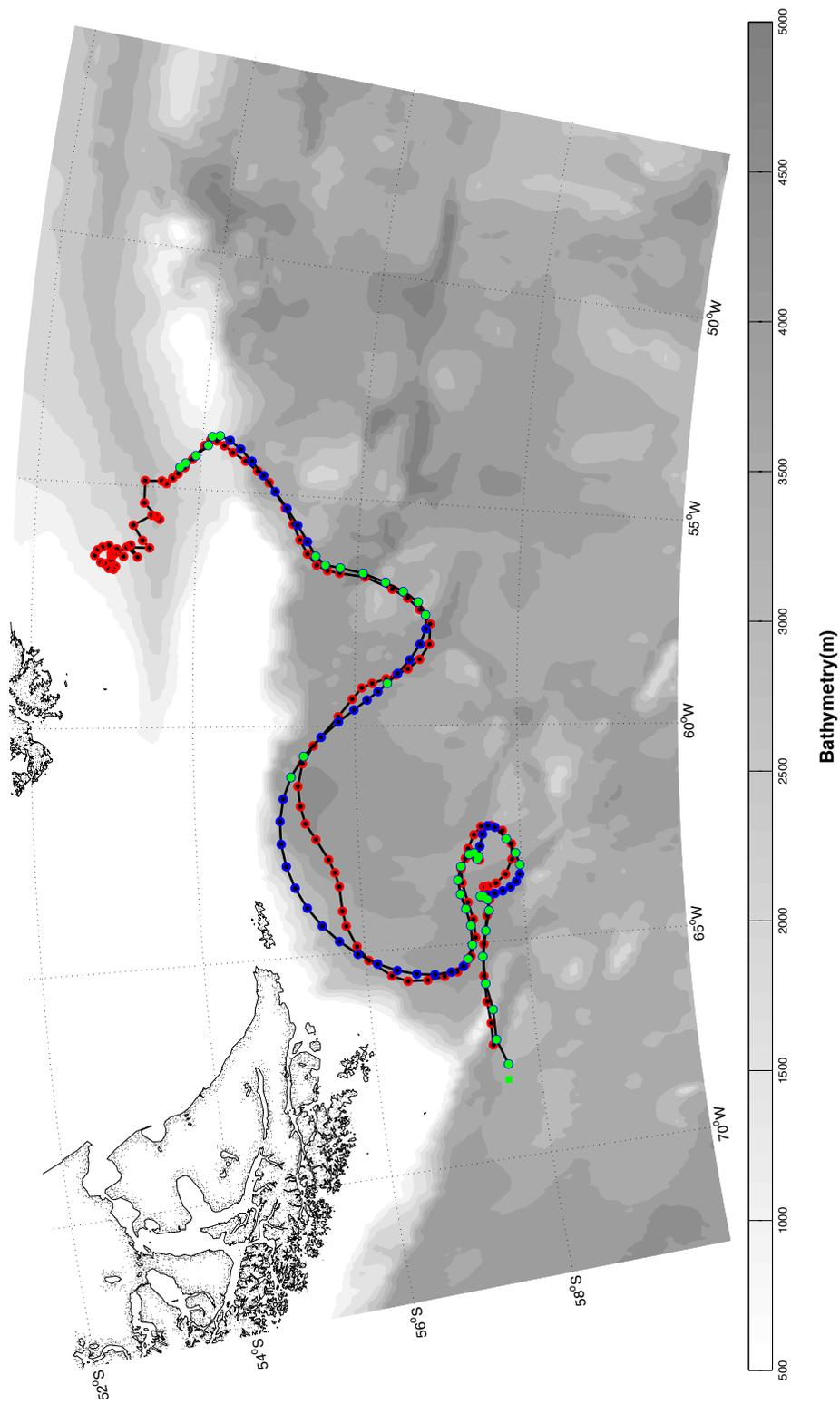
Figure 1b. APEX 4781 track diagram from sound source data (blue dots and line), GPS position (red dots and black line) and points of recorded TOA's (green dots). Bathymetry is shaded in 500-meter intervals, according to the color bar.
