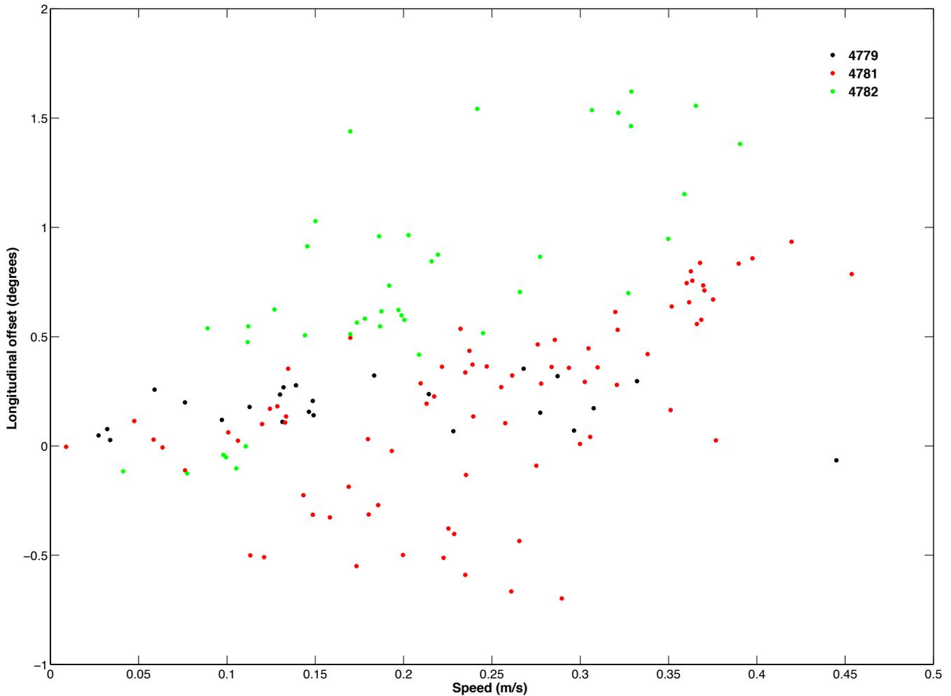
**Figure 7. Longitudinal offset (degrees) between ARTOA track and GPS position versus float speed (m/s) for APEX 4779 (black dots), 4781 (red dots) and 4782 (green dots). A positive longitudinal offset indicates GPS position is east of ARTOA track.**
