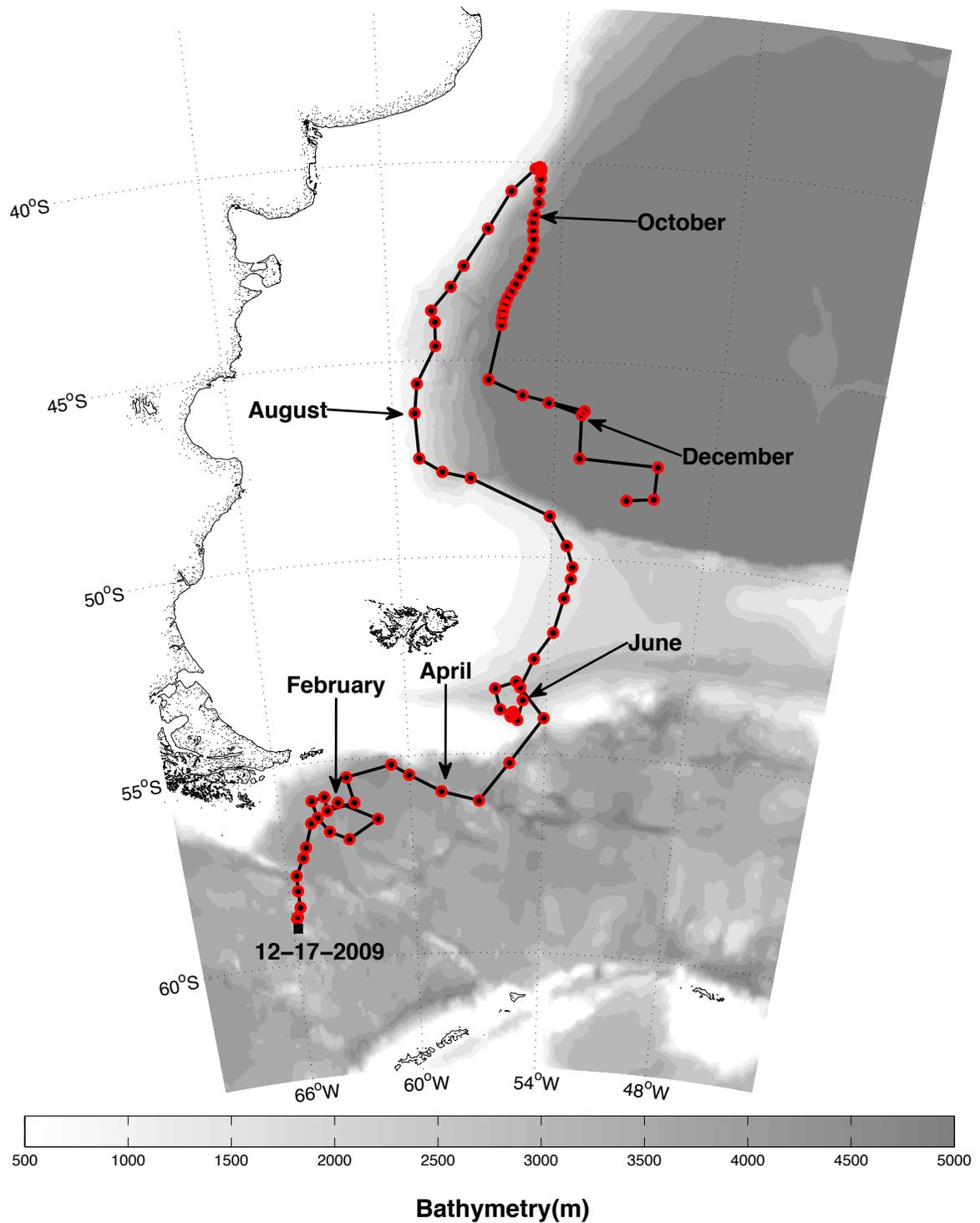
Figure 1a. APEX 4779 track diagram from GPS position data. Red dots indicate CTD profiles with GPS positions, whereas the black square is deployment position (with date). Bathymetry is shaded in 500-meter intervals, according to the color bar.
