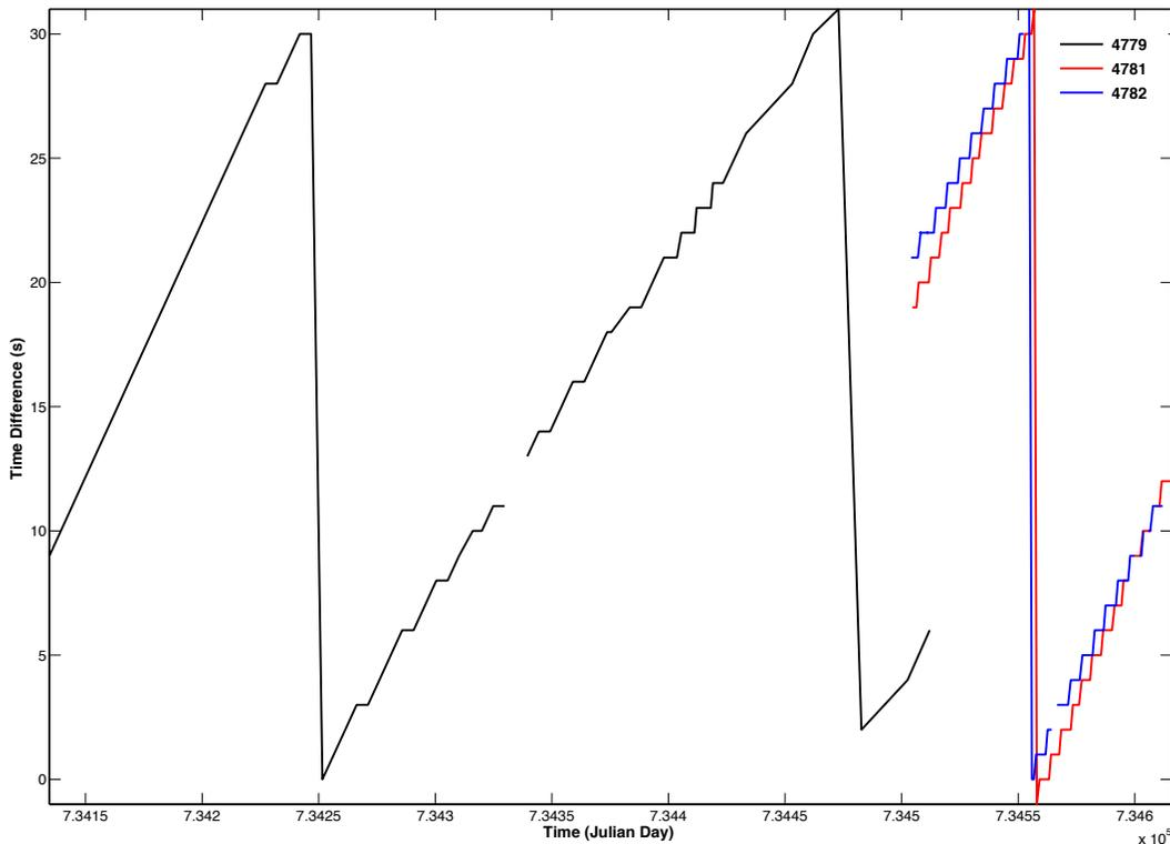
**Figure 6. Time difference between internal APEX clock and GPS time, for 4779 (black), 4781 (red) and 4782 (blue). If the time offset is excessive ( $>30$  s), the internal clock is reset to GPS time.**
