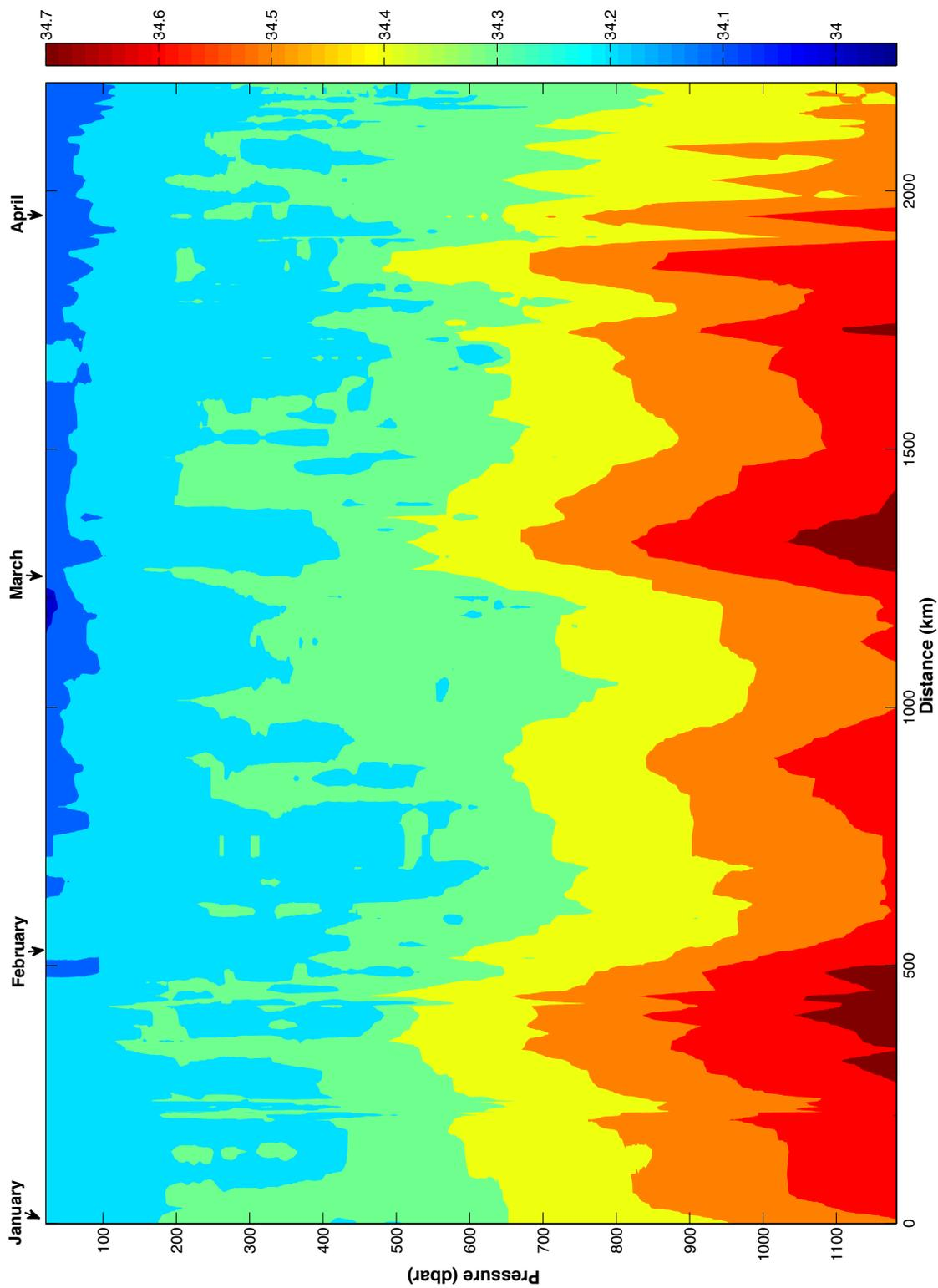
Figure 3b. Along track absolute salinity (g/kg) for APEX 4781. X-axis indicates horizontal distance (km) from the start of the section (i.e. first CTD profile).
