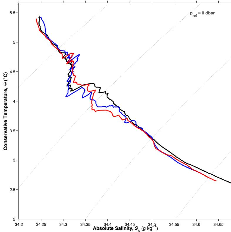
**Figure 5. Top: TS relationship for APEX 4779 profile 24 (blue), UK1 station 3 (black) and UK1 station 4 (red). CTD stations are ~59/66 km (respectively) east of the APEX profile, and sampled four months earlier. Bottom: TS relationship for APEX 4781 profile 2 (red), APEX 4782 profile 2 (blue) and UK2 station 42 (black). CTD station is ~55km west of APEX profiles, and sampled 2 days earlier.**
