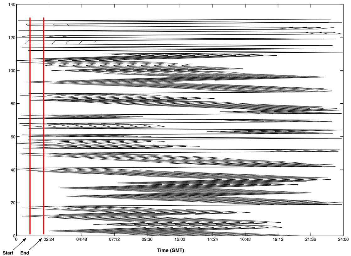
**Figure 3: Listening window (black lines) each day for APEX 4781 (top) and 4782 (bottom). The red lines indicate the start and end of the listening window. For a TOA to be registered, the black line must cross both red lines.**
