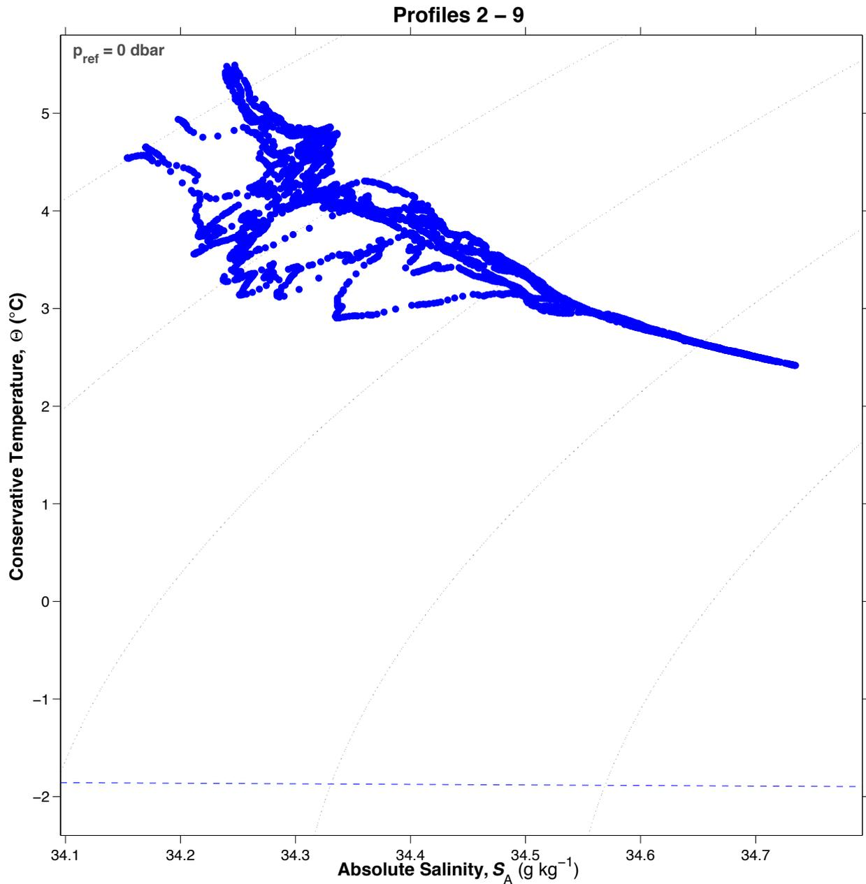
Figure 4: Conservative Temperature ( $^{\circ}\text{C}$ ) versus Absolute Salinity ( $\text{gkg}^{-1}$ ) along track, starting with the first profile after deployment, for APEX 4782. Each figure shows eight successive profiles. The freezing line is indicated by the blue dashed line.
