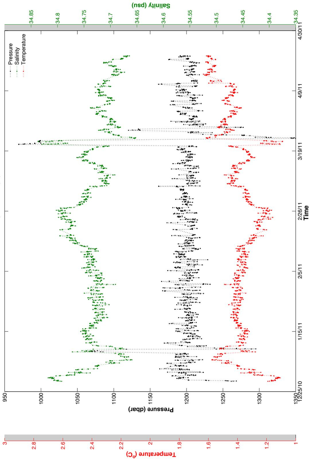
Figure 2. Pressure (black), temperature (red) and salinity (green) during the drift phase (~10-11 hrs) of each day for APEX 4782.
