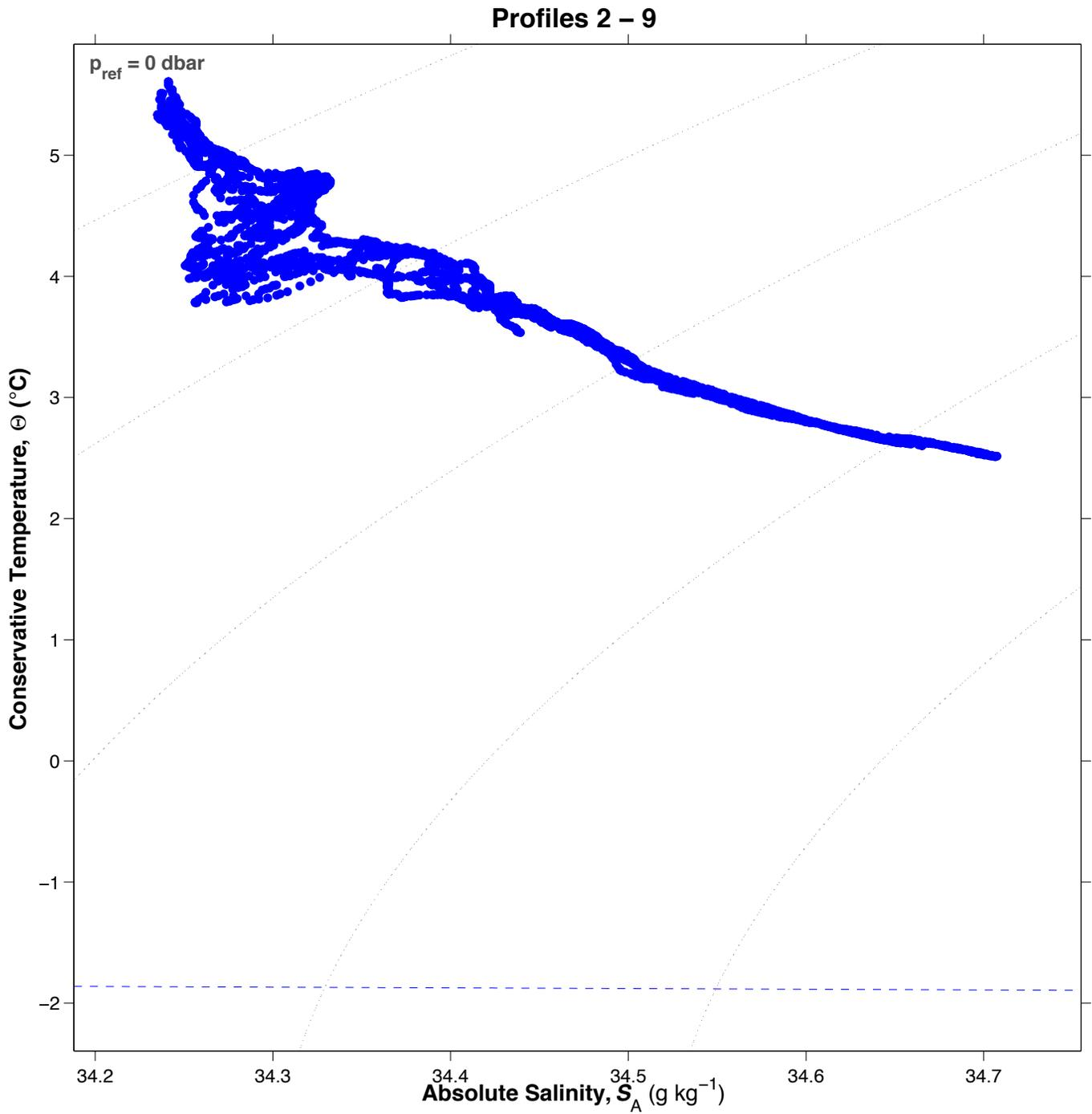
Figure 4: Conservative Temperature ( $^{\circ}\text{C}$ ) versus Absolute Salinity ( $\text{gkg}^{-1}$ ) along track, starting with the first profile after deployment, for APEX 4781. Each figure shows eight successive profiles. The freezing line is indicated by the blue dashed line.
