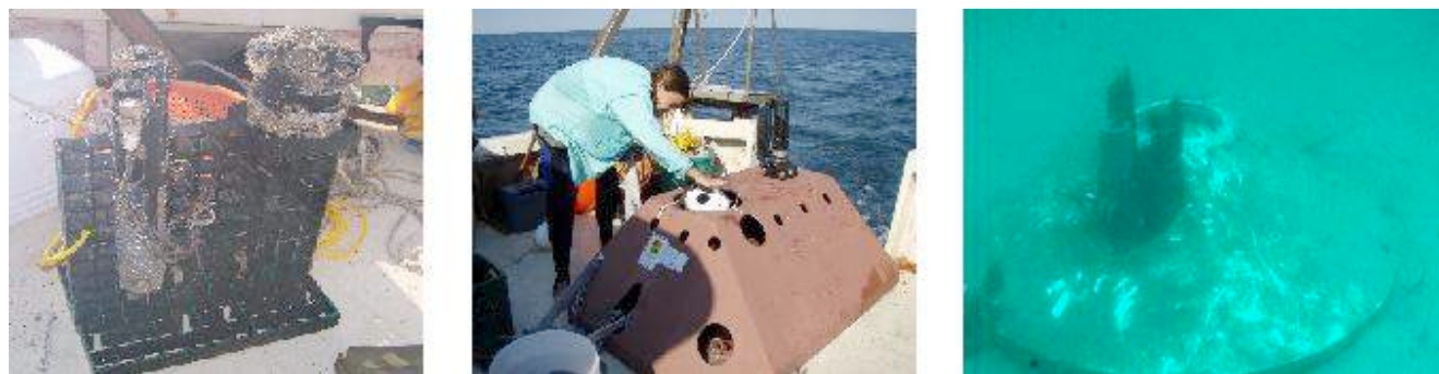
Figure 4. Left to Right: Site A bottom mount with AWAC and YSI after a deployment, Site B MSI bottom mount with a gimbed AWAC and YSI mounted in a custom hole, Site N7 MSI bottom mount with a gimbed ADCP and a custom basket with YSI, CDOM and Nitrate sensors.
