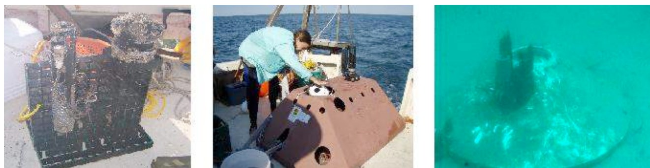
Figure 4. Left to Right: Site A bottom mount with AWAC and YSI after a deployment, Site B MSI bottom mount with a gimbed AWAC and YSI mounted in a custom hole, Site N7 MSI bottom mount with a gimbed ADCP and a custom basket with YSI.
